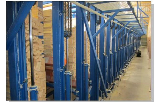
Box sorting line for boards and timber
