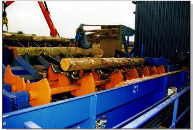
BRUKS Butt reducer in a Brødbæk & Co. line
