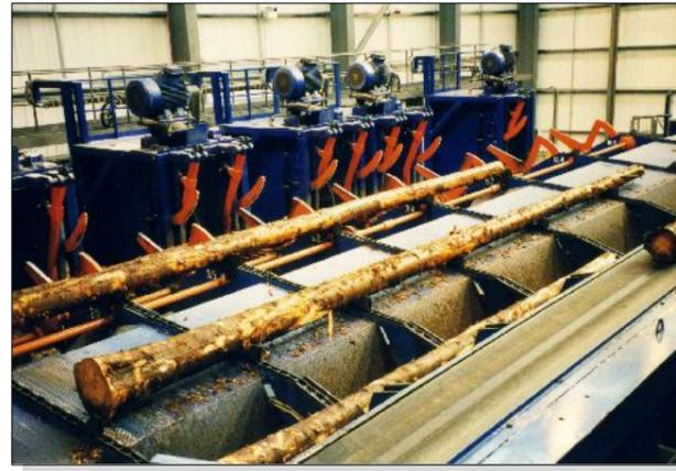
High capacity cross-cutting line for long poles
