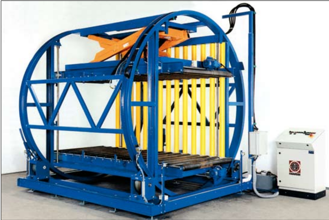
Stack turner for turning of whole pallets with parts.
