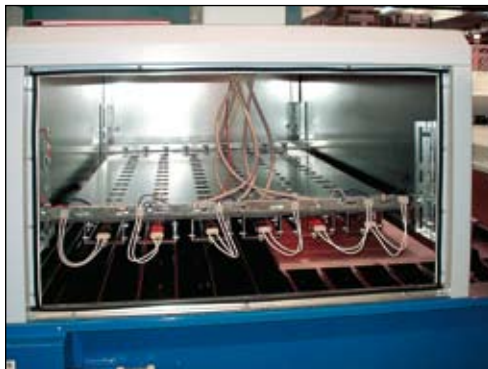
Detail of the speed dryer showing the jets and placement of IRM curing lamps.
