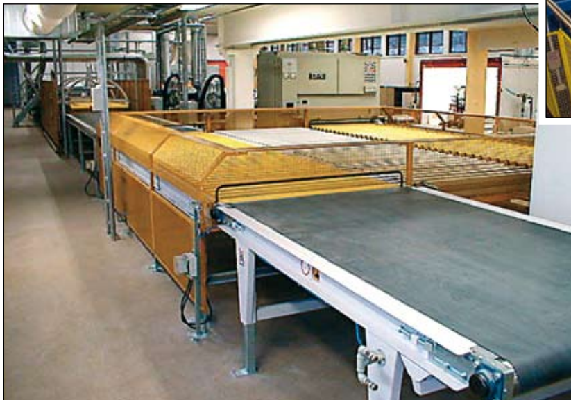
Double angle transfer for 180 degree turning of parts, integrated panel turner in the top.
