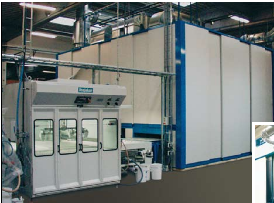
Vertical dryers are suitable for drying of lacquers with long evaporation time and high content of solid matters, e.g. water based lacquers and PUR-lacquers.
