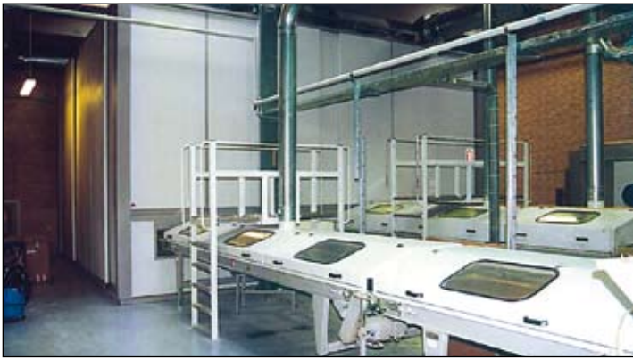
Above picture shows a horizontal path system for lacquering and drying of inside ceiling panels.
