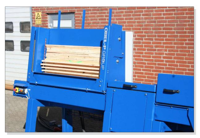
Infeed magazine for a stack of random width boards. At the bottom is the infeed chain with steel dogs, for a positive feeding of even wet boards.
