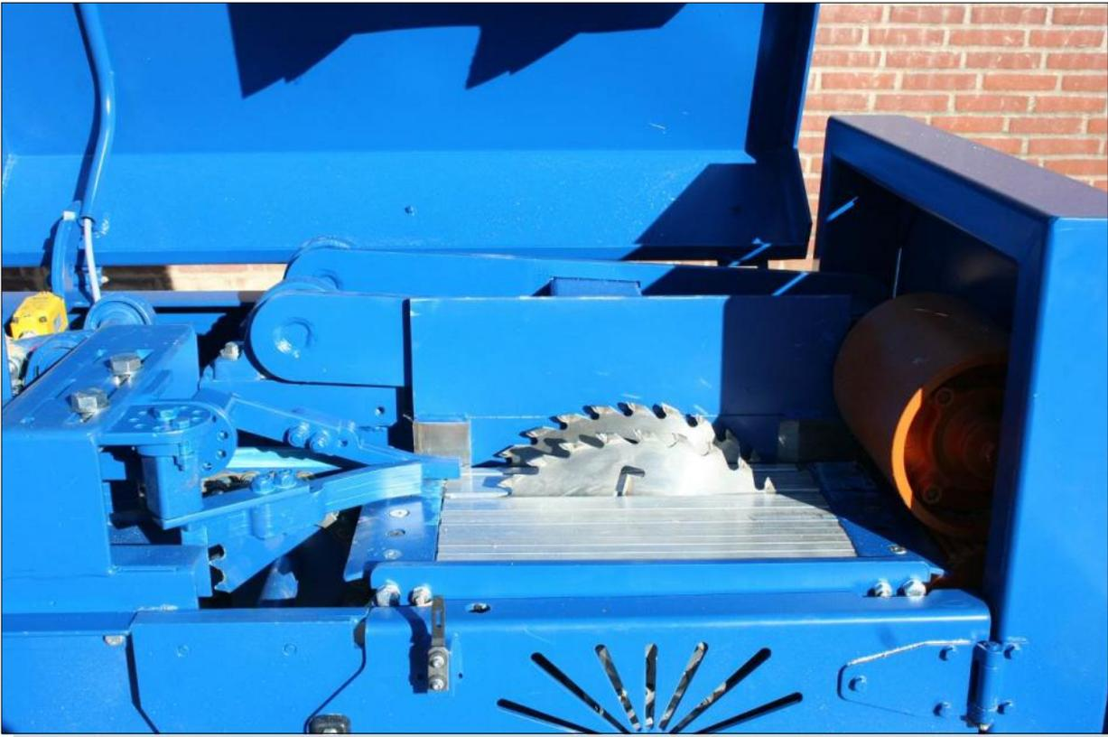
The basic Stick App unit with a vertical saw for cutting boards and sticks.
