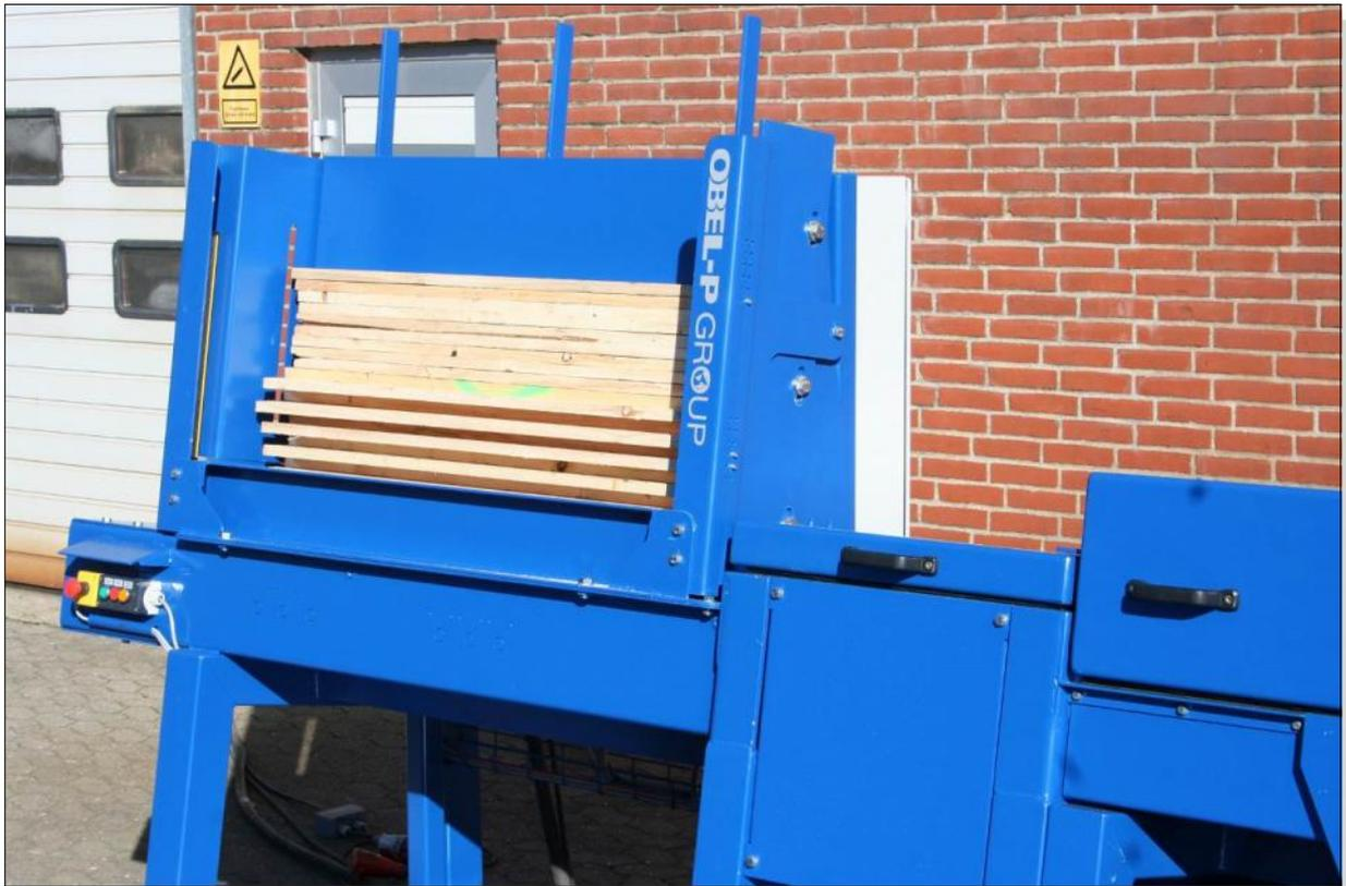
Infeed magazine for a stack of random width boards. At the bottom is the in-feed chain with steel dogs, for a positive feeding of even wet boards.
