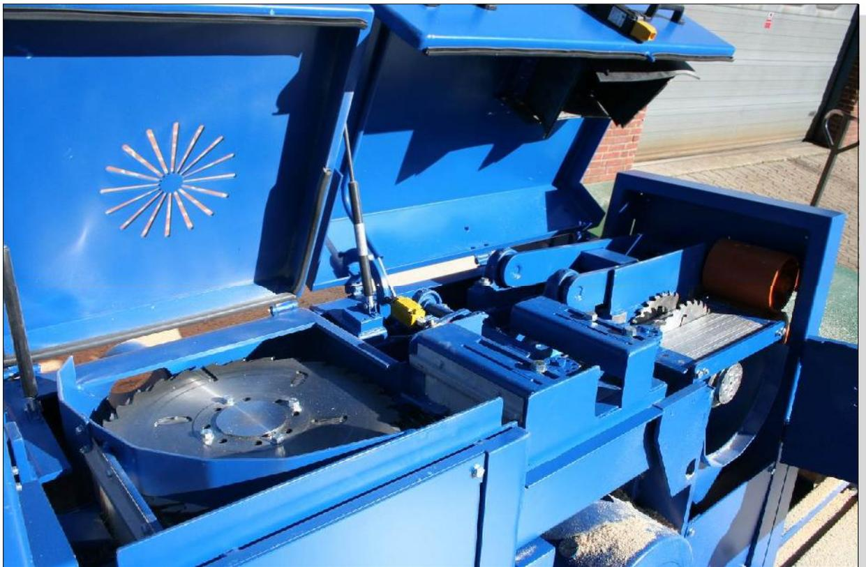
To the left is the StickApp Plus unit with a horizontal saw bush for calibrating the thickness of boards and sticks.
