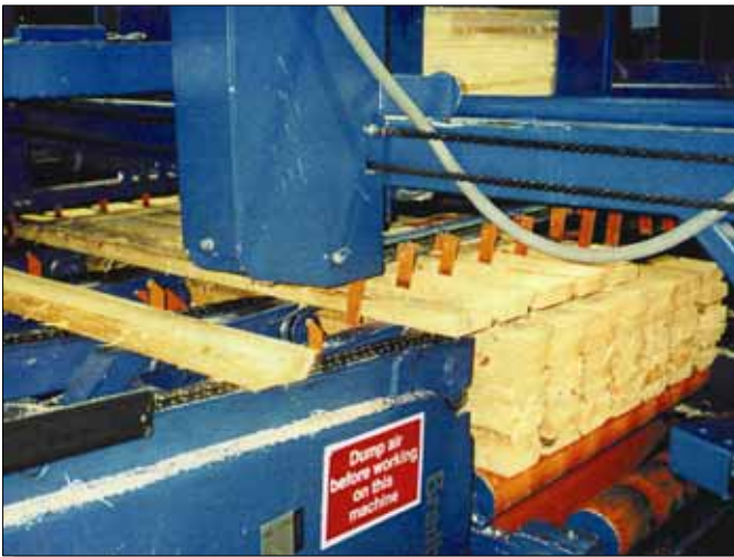
20. Slat stacking, 5 mm thick
