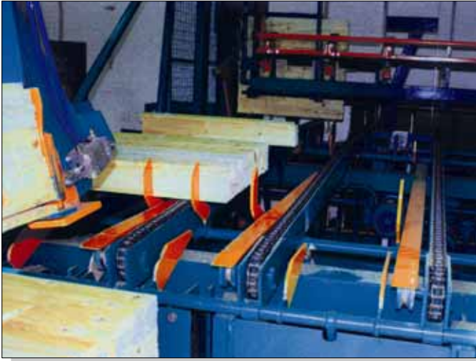
18. Multi layer stacking – 500 boards/min.
