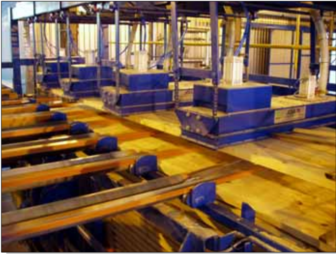
12. Vacuum destacking – very fast process
