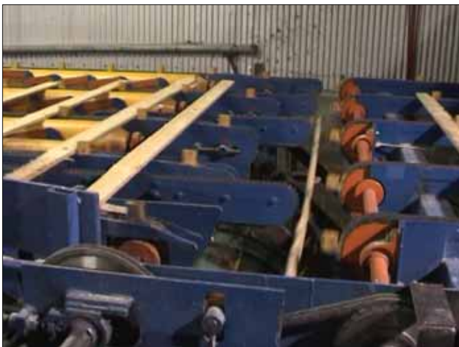
3. Dump gate before trimming
