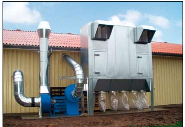
Rotary valve filter and bag filter systems, we can always find a solution corresponding to the demands of the customers.
